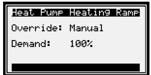
Figure 9 - Reversing Valve. Change override to manual and demand to 100%.
