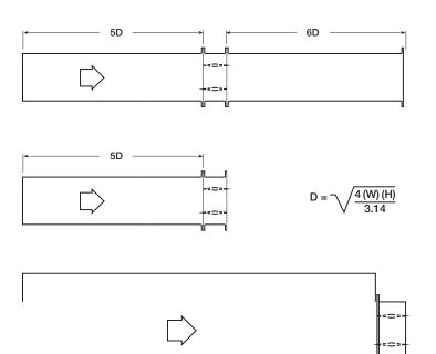
D = Duct lengthW = Damper widthH= Damper height
