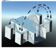
\* The Greenheck model IDHE duct heater is universally configured to allow airflow in either direction in all mounting orientations.
