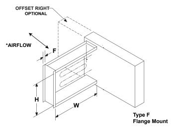
\* Greenheck duct heaters are universally configured to allow airflow in either direction in horizontal ducts.
