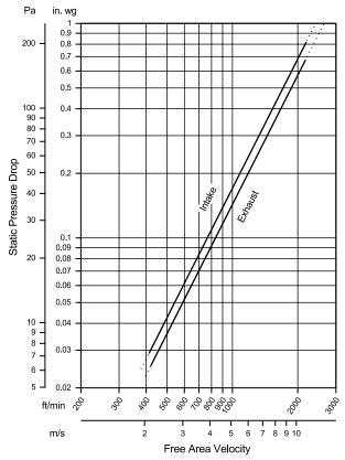
Model ECD-401 resistance to airflow (pressure drop) varies depending on louver application (air intake or air exhaust). Free area velocities (shown) are higher than average velocity through the overall louver size. See louver selection information. (Test Figure 5.5-6.5)
