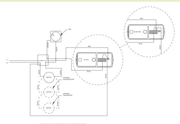
1. CONDUIT RUNS WHICH EXCEED 72" MUST HAVE GREEN GROUND WIRE.
