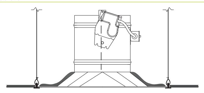
This is a typical Lay-in Diffuser application. See installation instructions at www.greenheck.com for more application information.
