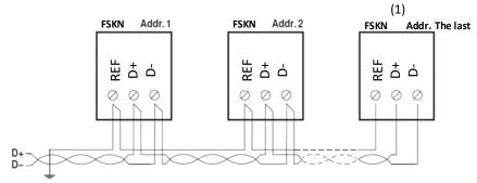
The wiring of the line for BACnet MS<sup>/</sup>TP or Modbus RTU must be carried out in accordance with applicable RS 485 standards·
