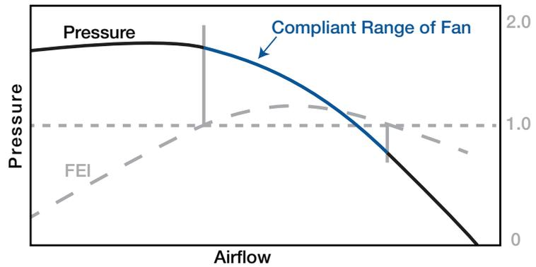
Figure 3: Compliant range of operation of a fan operating at multiple speeds
