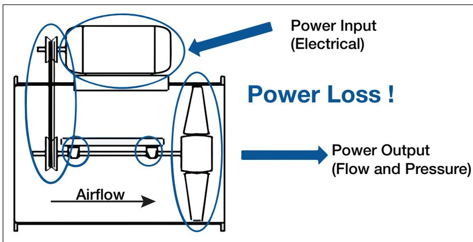
Because the actual and baseline powers are obtained (calculated) at the same airflow and pressure, FEI is also defined as the ratio of Actual Fan System Efficiency to Baseline System Efficiency. (Equation 2)
