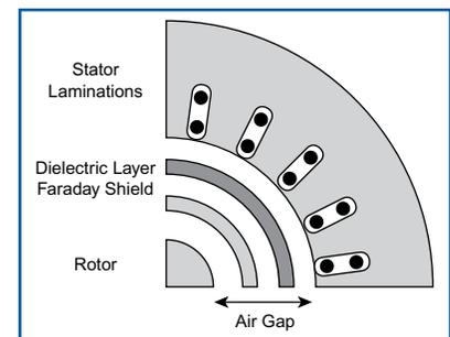
*Electrostatic Shielded Induction Motor (ESIM) with Faraday shield*
