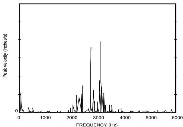
*Example of vibration spectrum showing “Bearing Fluting”*
